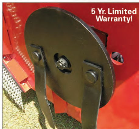
SOLID STEEL STUMP JUMPER Round • 3/4" thick
