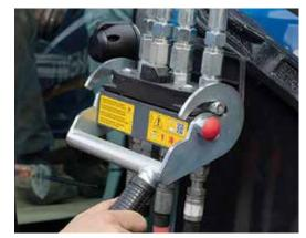
2 With the Hydro-Fix all hydraulic lines can be connected to the tractor at the same time. The front loader is lifted slightly to hold the locking pin in position in the catch hook of the connection support.
