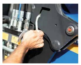
The locking lever is pressed downwards and the front loader securely held in position on the attachment component. Then the front loader is raised higher.
