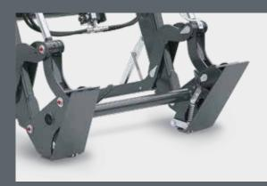
The Skid Steer quick release frame provides a clear view of the implement – ideal when working with the bale spike or pallet fork.
