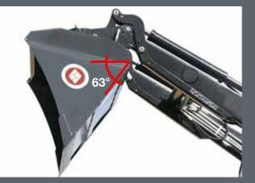
Then the bucket is completely empty – the dump angles for the implement provide efficient results.
