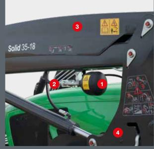
The Comfort-Drive is protected between the drive-in column and the lifting arm bar. It can be switched on and off with the stopcock.
