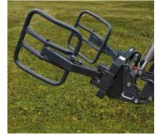
Tilt the implement - the locking mechanism automatically slots into place.
