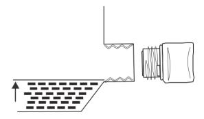
Figure 4: Engine Oil Correct Level
