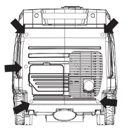
Figure 20: Remove Muffler Access Panel
