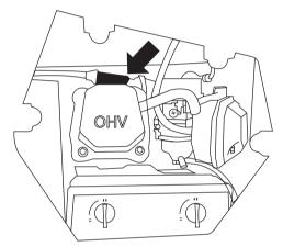
Figure 18: Pull off Spark Plug Cover
