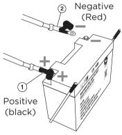
Figure 2: Installing Battery Leads
