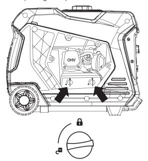
Figure 14: Unlock Air Filter Cover
