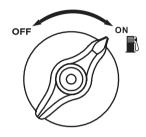
Figure 7: Turn Fuel Switch to ON Position
