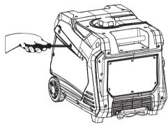
Figure 13: Remove Engine Service Panel
