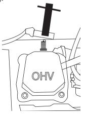
Figure 19: Remove Spark Plug
