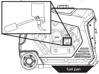
Figure 17: Loosen Float Bowl Screw
