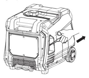
Figure 9: Pull the Recoil Handle out from Inverter 7.
