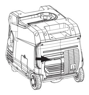
Figure 1: Battery Service Panel
