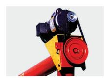
Portable 4" auger, adjustable motor mount, shielded single "A" belt and pulley, and pre-lubricated top end bearing.
