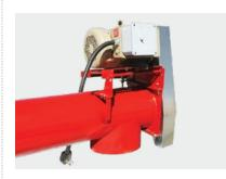
Upper drive has heavy-duty flangette ball bearing and adjustable motor mount with double "B" belts and pulley (triple belts on 13" models).
