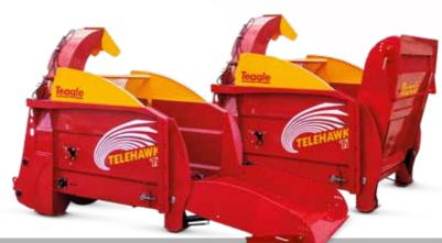
Introducing the new **Telehawk T2 Straw Bedder** now featuring a hydraulic loading gate for even easier self-loading, improved bale processing and greater manoeuvrability. Also now featuring an enhanced crossbeater design for **improved driveline** protection against foreign objects in the straw.
