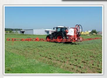
**TANK:** from 1300 to 1900 l **BOOM:** from 14 to 24 m
