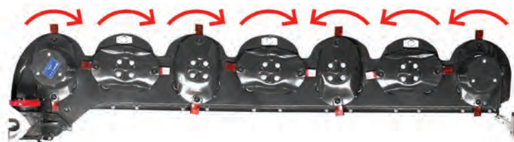
Disc rotation towards the centre provides a narrower windrow when mowing on extremely steep terrains.
