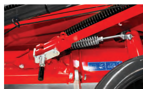
The lock of the mower in the parking position prevents the drop of the linkage due to pressure in the cylinder and allows simple attachment to the tractor.
