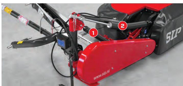
DUAL SPRING suspension system. The first spring (1) relieves the inner heel, and the adjustable second spring (2) relieves the outer heel of the cutter bar. The system enables the sequential lifting of the cutter bar, thus preventing damage to the turf.
