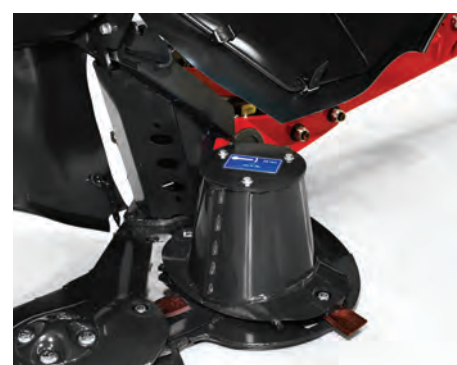
The drive via the gearbox placed behind the first disc prevents forage from accumulating inside the cutter bar.
