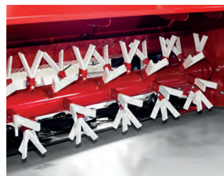
Finger plastic conditioner (FPC) for optimal conditioning of grass-based forages with the possibility of conditioning intensity adjustment.
