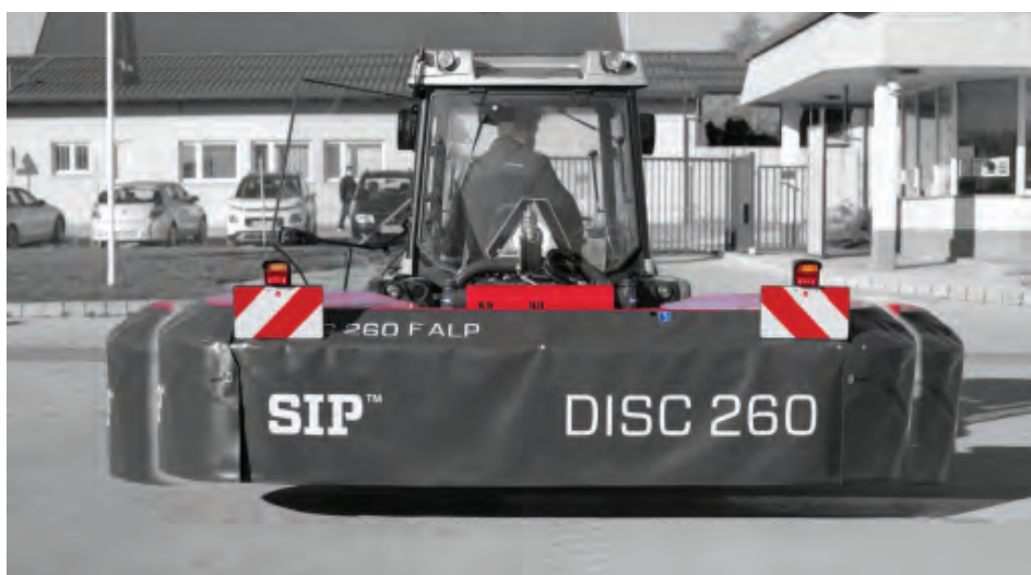
The hydraulic side shift (optional) allows the mower to be shifted 200 mm to the left or right and ensures consistent forage flow between the tractor wheels even when working on a slope. The lateral adaptation to the ground is \pm 10^\circ .
