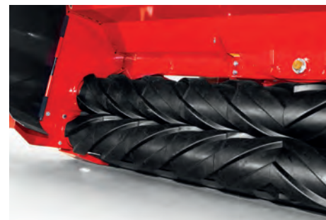
The roller rubber conditioner (RRC) enables evenly conditioned alfalfa and clover forage. Conditioning intensity is continuously adjustable.
