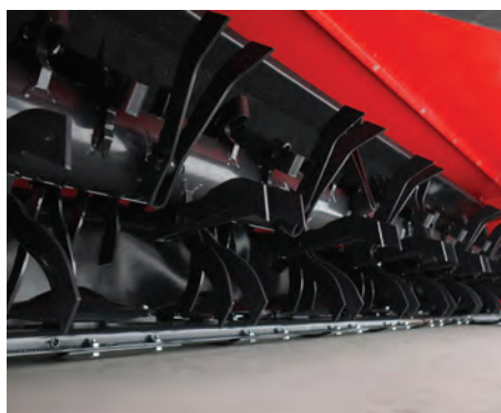
Flexible steel fingers damage, break, and "shred" the stems, thus allowing fast moisture loss.
