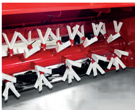
Rigid plastic fingers scrape and damage the epidermis on the stems and leaves and break the stems.
