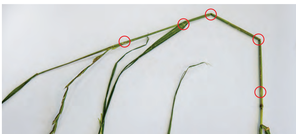
The picture shows the points where the finger conditioner damages the epidermis and breaks the stems.
