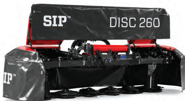
The wide opening of the cutter bar cover enables easy maintenance and cleaning of the mower.
