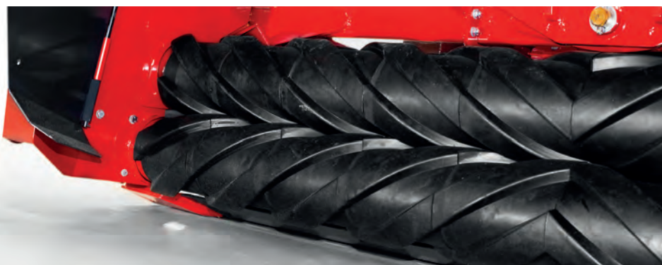
The profiled helix-shaped rubber rollers rotate against each other and compress stems lengthwise, allowing quick moisture loss.
