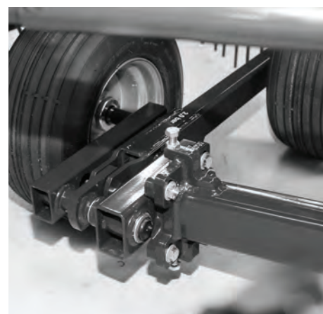
Rotor angle adjustment for a cleaner swath.
