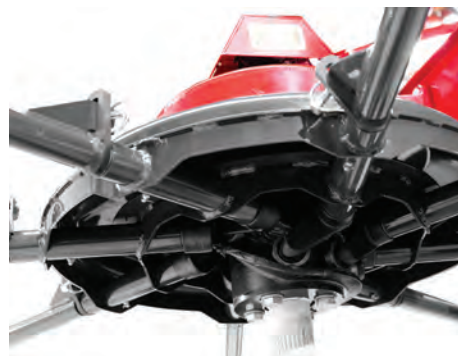
Cam track made of ductile iron.
