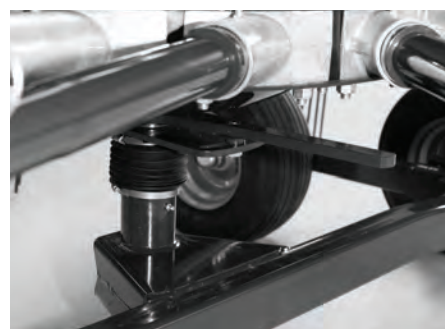
Adjustable cam track \pm 15^\circ depending on the quantity and moisture of the forage.
