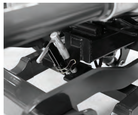
Easy and simple rotor height adjustment with a threaded bolt.
