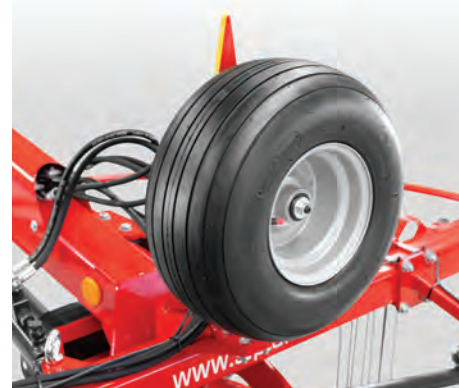
Spare wheel on the back of the machine as part of the standard equipment.
