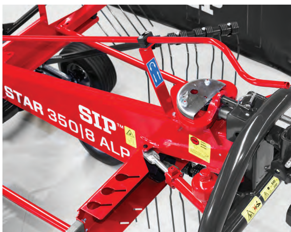
The working height of the spring tines is easily adjustable from the tractor.
