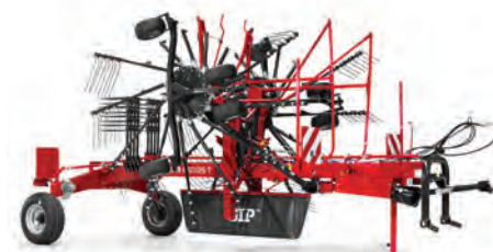
The transport height of all models is below 4 m. With folded protections and spring tine holders, it is between 3.2 and 3.5 m.
