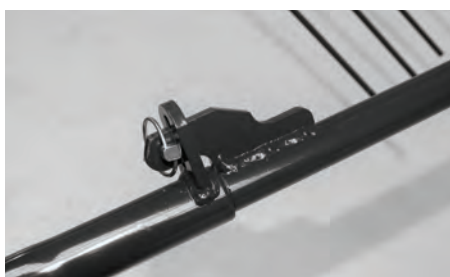
Rotor angle adjustment for a cleaner swath.
