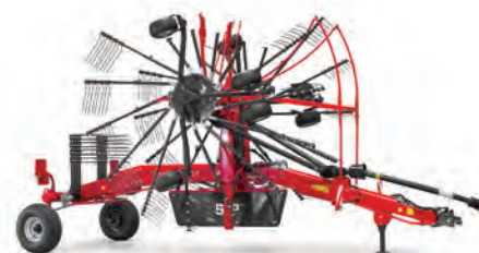
The transport height with folded protections and spring tine holders is 3.99 m.
