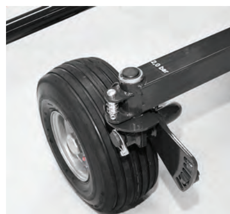
The walking tandem axle (SIP patent) enables optimal adaptation to terrain, higher working speed, and transfer of lower loads to the machine (STAR 350 | 8 ALP).
