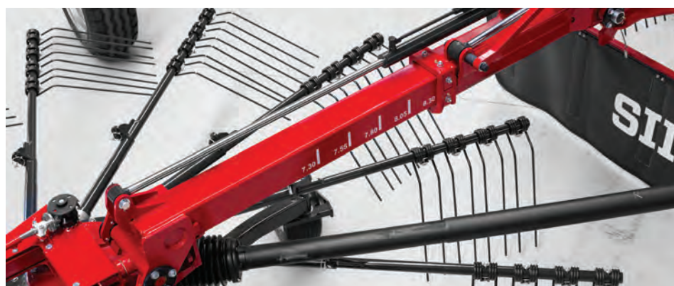
Hydraulic continuously adjustable swath width (standard with STAR 850 | 26 T, optional with 72022 T and 650I20 T).
