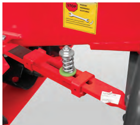
Additional mechanical shock absorber (available with STAR 320|8 ALP, 350|8 ALP).
