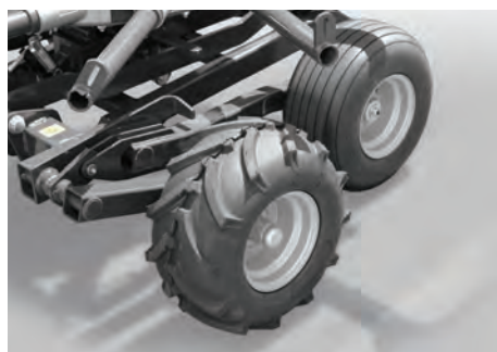
Wheel with tractor profile (available with STAR 430|12 T, 600|20 T)
