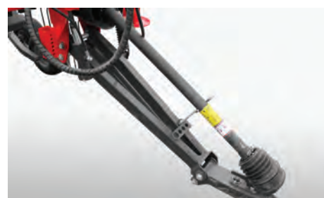
The hitch ring is controlled by parallel linkage. The hydraulic arm on the drawbar maintains the leading rotor parallel to the ground as it is lifted and lowered.
