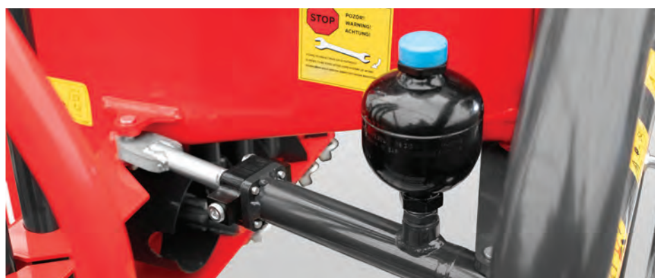
The additional hydraulic shock absorber enables easier following of the tractor (optional at STAR 320 | 8 ALP, 350 | 8 ALP).
