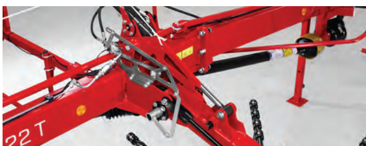
The sequential lift of the rotors (TAKEOFF) via a one-way hydraulic connection ensures excellent manoeuvrability and easy operation.
