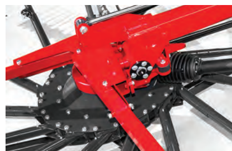
Robust 3D pivoting hinge in front of the rotor.
