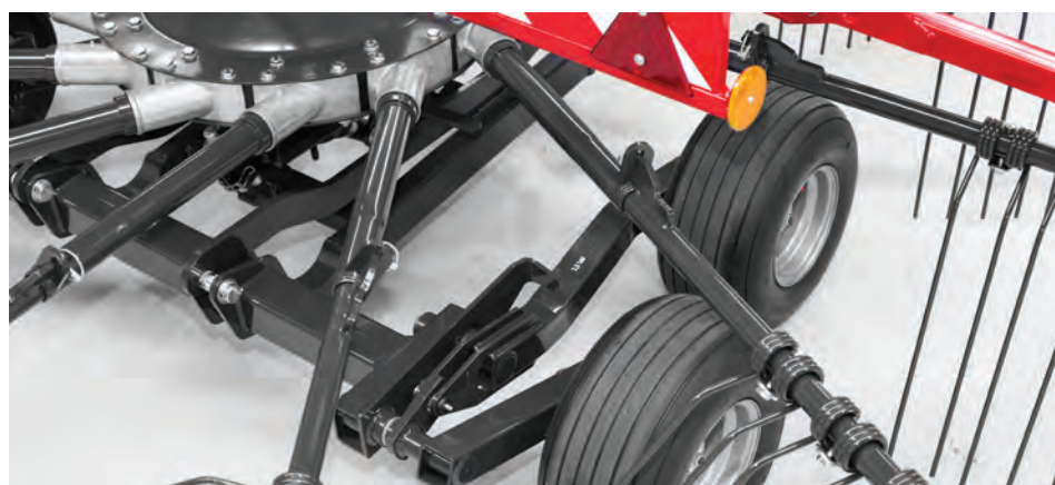
The front rotors are equipped as a standard with a SIP walking tandem axle (SIP patent), which enables optimal adaptation to terrain, higher working speed and lower load transfer to the machine.
