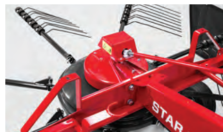
Working height is adjustable from the tractor.
