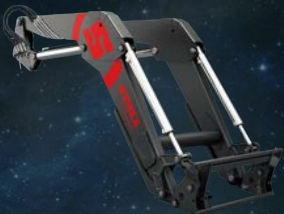
FS lifting arms without parallel linkage: For tough jobs with the best price-performance ratio.
