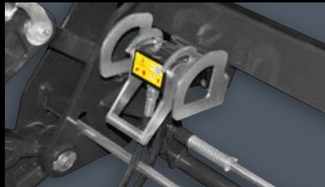
TOOL FIX. 1-way coupling for the 3rd pilot circuit.
