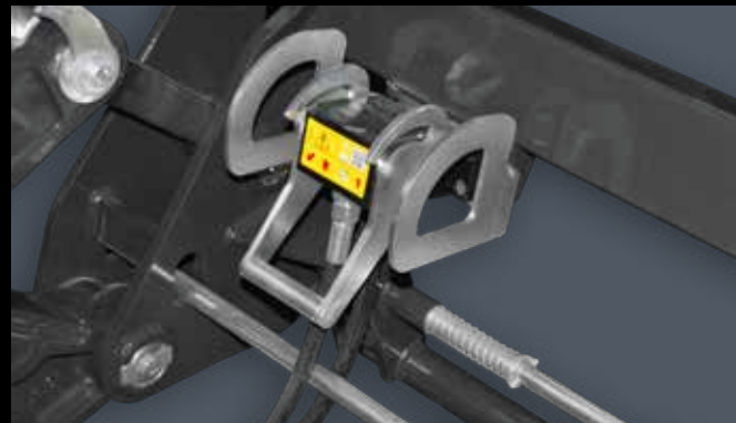
TOOL FIX. 1-way coupling for the 3rd and 4th pilot circuit.
