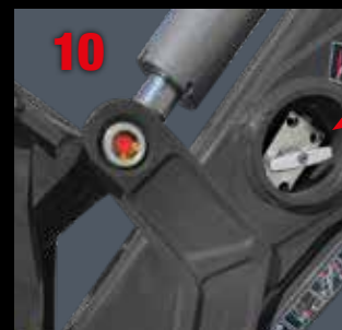
NEW: Switch lever on the left side of the lift arm.
