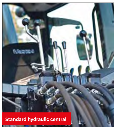
Light 2-lever control with on/off switches
